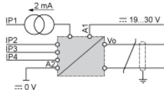
The input, output and power supply lines must be kept away from the power cables to avoid effects due to induced interference.
